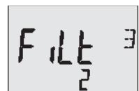
(Filter 0 → no damping, Filter 3 → max. damping)
