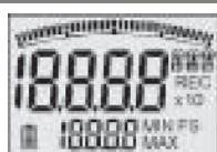
A self-test procedure is carried out
