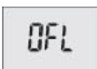
This indicates that the applied pressure is outside of the full scale range.
